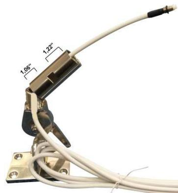
4. Screw the FME connector onto the base of the antenna until hand tight
