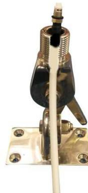
3. Pass the RG-8X cable through the lower part of the ferrule. Pay attention: put the shortest part of the lower ferrule on the mount as shown on the picture
