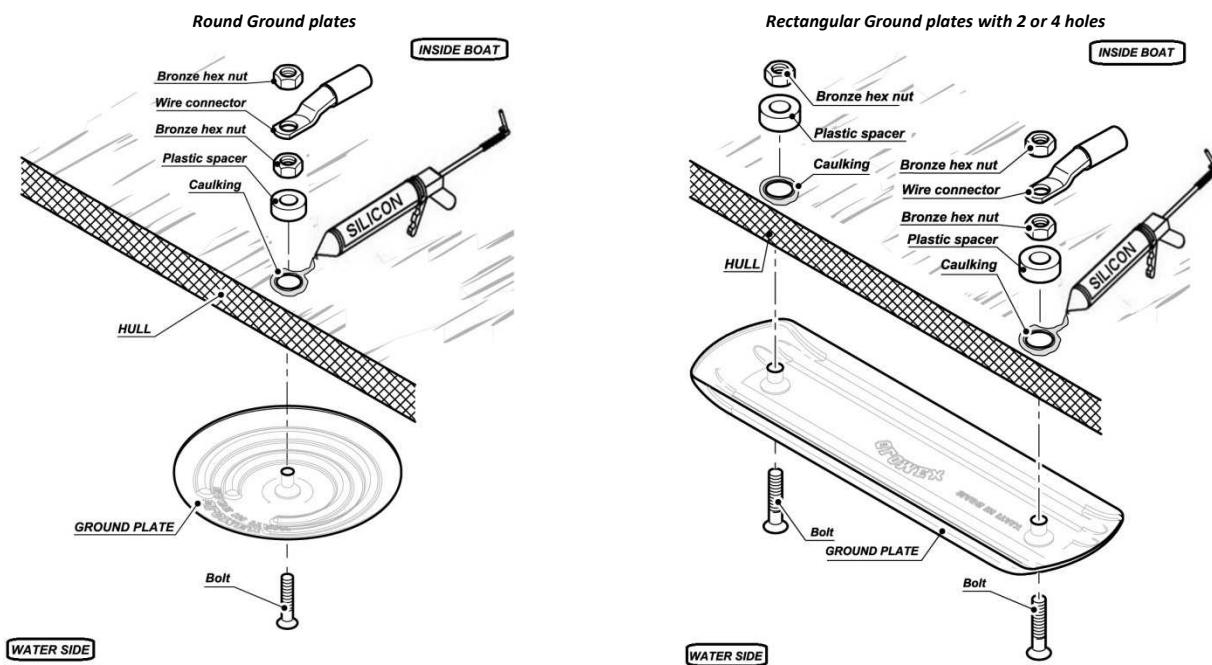
1. Clean and dry the inside surface of the hull around the mounting location. It is very important to remove any grease or oil that could prevent the caulking to adhere to the hull.
