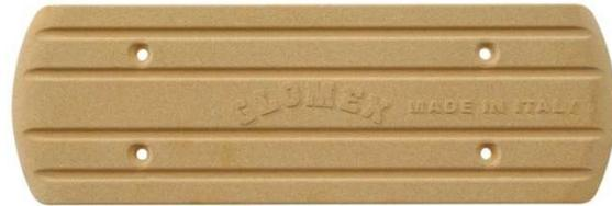
**RA207** - 455x150x13mm (18x6x1/2"). Ground equivalent Surface: 5,75 sq/mt. *Supplied with 4 screws, 4 spacer and 5 nuts - Use: 2 plates for SSB 800W (or more)*
